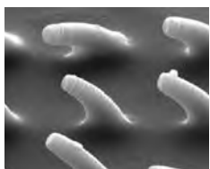
Posts moved by hydrogel 2,000 nm wide
